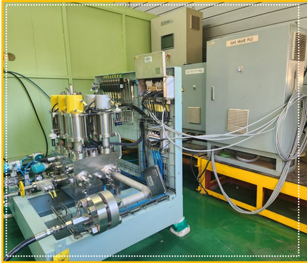
GVT (Gas Valve Train) Test Facility, Design pr': 420bar, Fluid : N 2 , Size 1~2"
