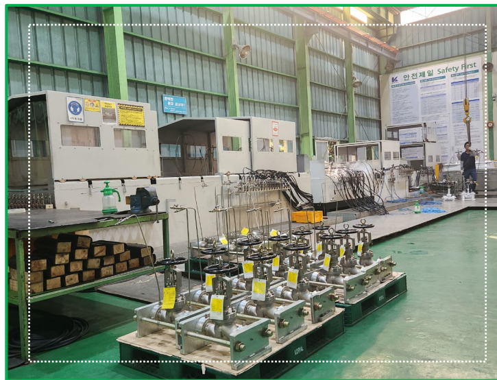
Cryogenic Test Chamber, ½" ~50", We can carry out 1 lot 50sets valve
