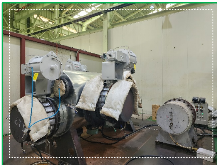
High Temperature Test Facility, Up to 600'c, 5set VV's can be tested simultaneously
