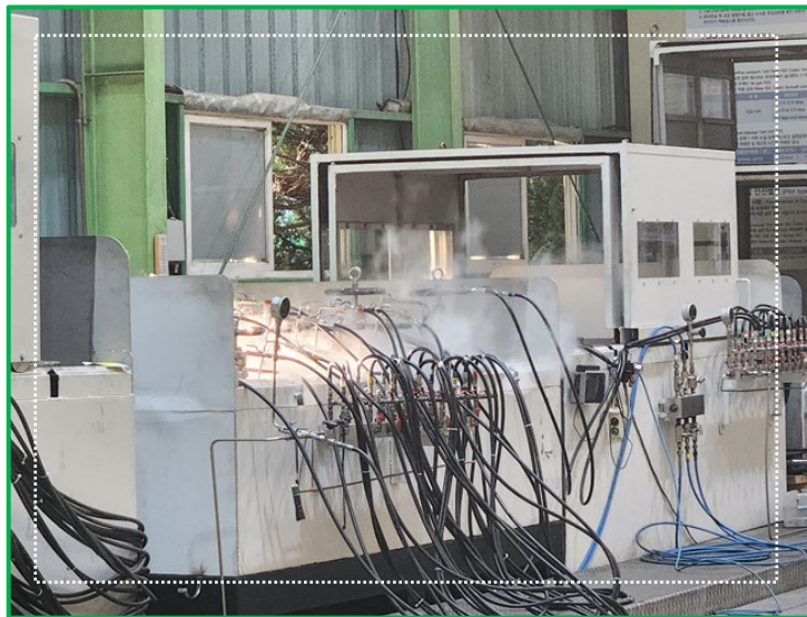
Cryogenic Test Chamber, ½" ~50", We can carry out 1 lot 50sets valve
